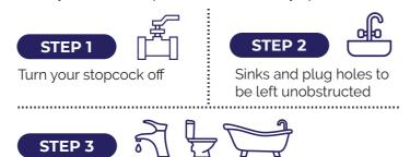
Ensure all water taps are left open/on, plugs are removed from plug holes, water is emptied from cistern and sinks/showers/bath
